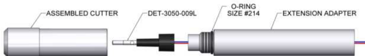
Figure 3: Exploded Arming View of Tubing Cutter Using DET-3050-009L
