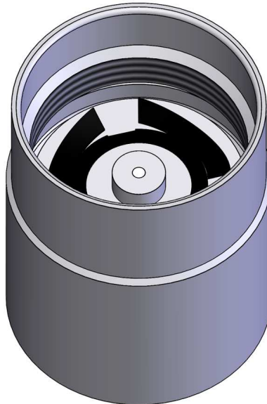
Figure 6: Finger Spring Washer Installation
