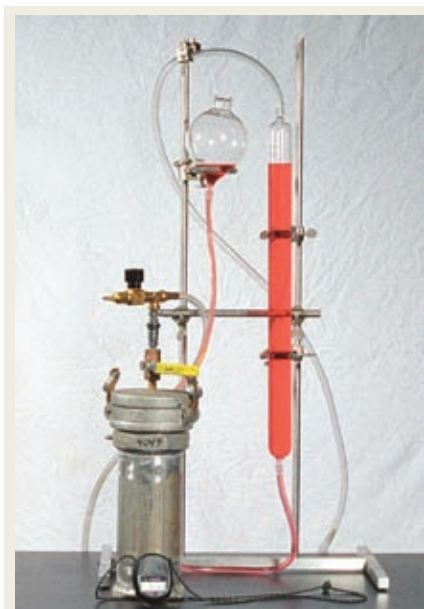
Fig. 1. Typical gas desorption canister, barometer and burette. Burette size varies according to expected gas volumes.
