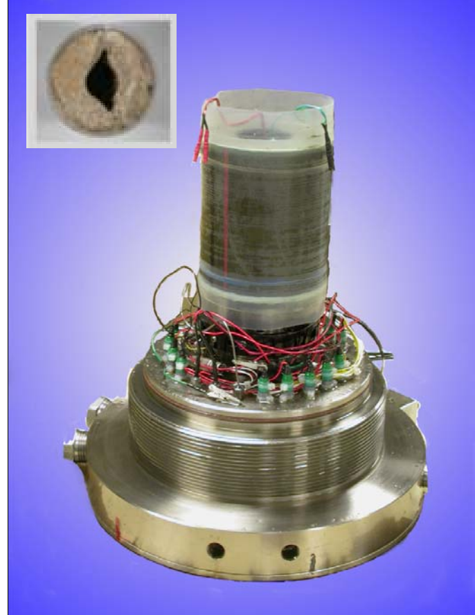
Whole core sample after advanced thick-wall cylinder test. (inset)
