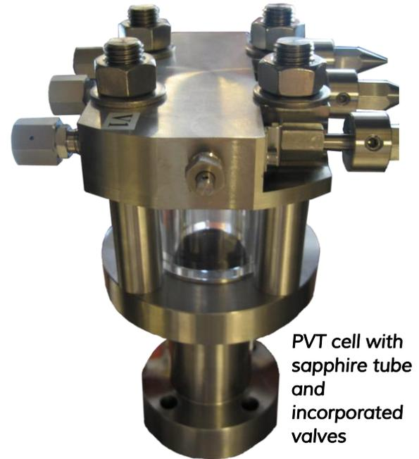
PVT cell with sapphire tube and incorporated valves
