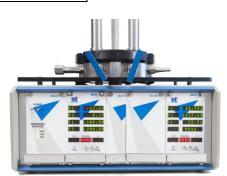
All wetted parts are made of Stainless Steel (ref SS316) except the tube (Glass) and the piston (Gas Resistant Plastic)
