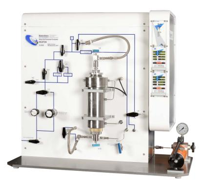
The MG2P is designed to measure steady state gas permeability, Klinkenberg and Pulse Decay permeability, pore volume and grain volume at room conditions.
