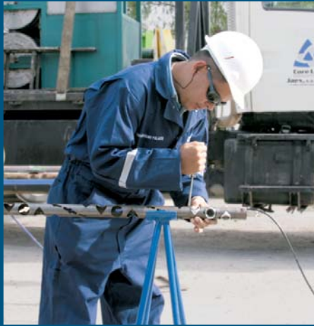
Felipe Lom prepares a HERO perforating gun system for deployment.
