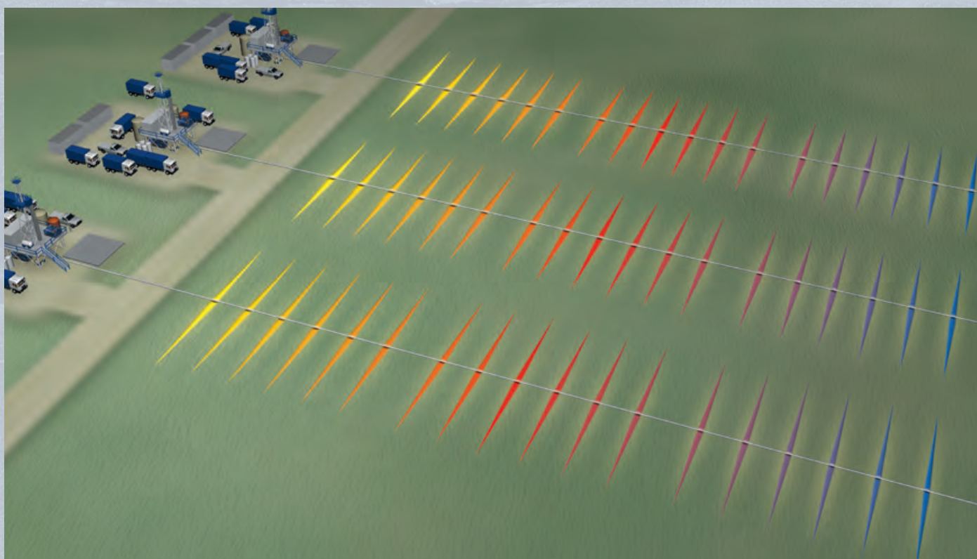
Figure 8. Multi-staged simul-fracs from pad drilling expand the surface area of the shale that can freely flow hydrocarbons into the fracture system.
