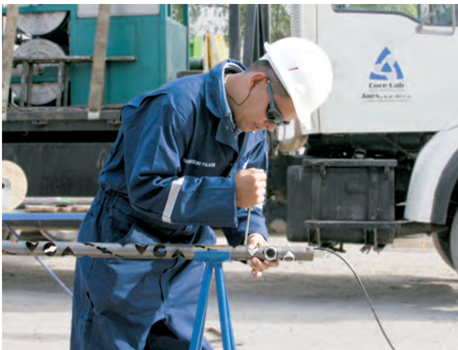
A Core Lab engineer preparing a perforation gun with charges and setting up for downhole deployment.
