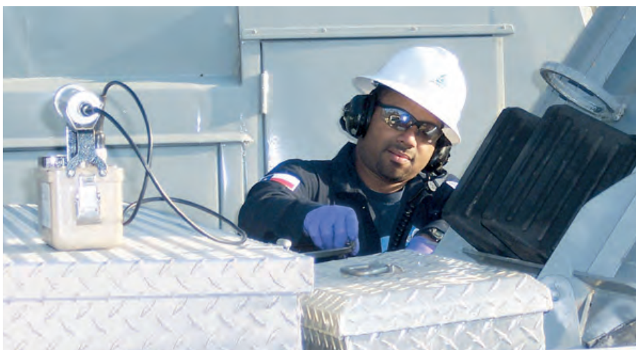
A field engineer setting up the equipment to inject SpectraChem tracers into a tight-oil well.
