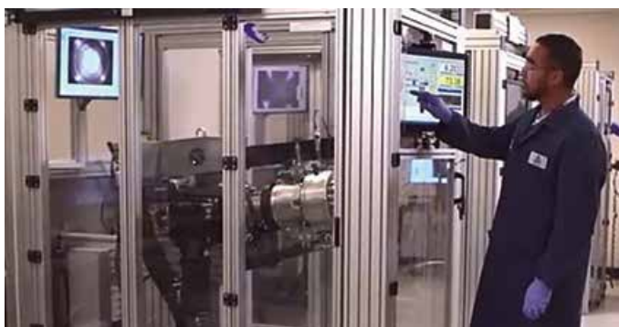
Figure 5. An automated HP/HT PVT cell.
