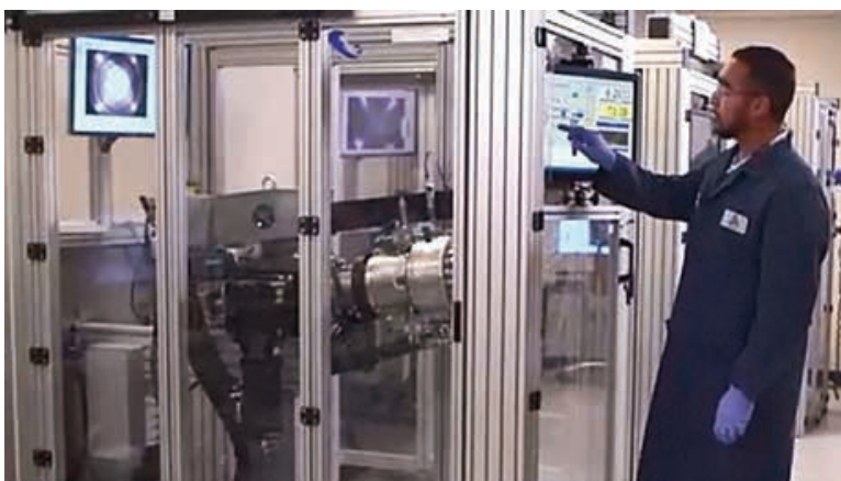
The Core Lab HP/HT PVT cell can test live reservoir fluids at pressures to 29,000 pounds per square inch and temperatures exceeding 390 degrees Fahrenheit.
