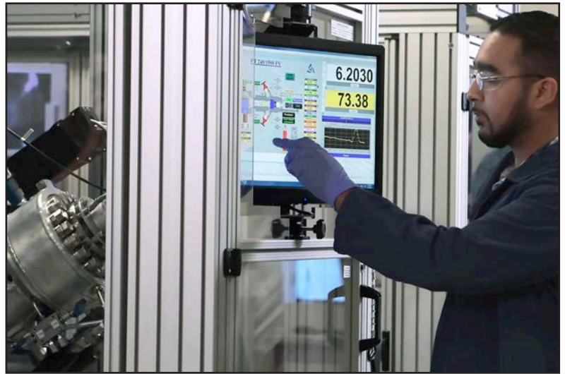
The Core Lab HP/HT PVT Cell can test with full visibility live reservoir fluids at 250 ml and 2000 bar
