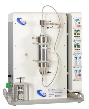
The AG2P is an automatic and highly accurate system for determining rock properties such as permeability, Klinkenberg permeability, pore volume, porosity and grain volume at overburden pressure. The system uses an unsteady state pulse decay technique for the permeability measurement.
