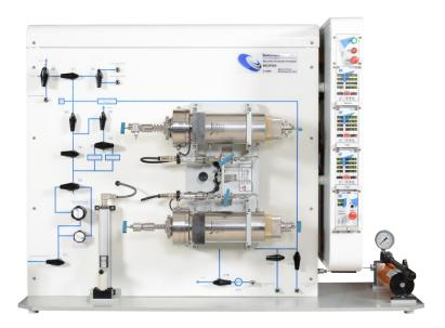
The MG2P 2R is designed to measure steady state gas permeability, Klinkenberg and Pulse Decay permeability, pore volume and grain volume at room conditions.
