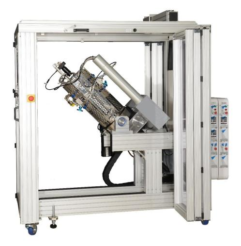
Our Reservoir Fluid PVT Analysis System composed of one set of PVT instrument (PVT 250/1500 full visual 250cc) and some ancillary equipment, as gasmeter, HP pressure sample cylinders, viscometer, etc.is able to perform analysis of different GOR reservoir fluids as crude oil, volatile oil, gas condensate and gas under high pressure and temperature conditions.
