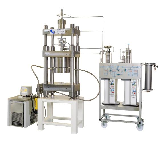
To continue the development of its range of triaxial press, ST has designed a press for solid deformation study working under high pressure and high temperature. The sample already preinstalled in a vessel is loaded in the center of the press. A unique jack gathers together three concentric pistons applying three different pressures: prestressed pressure, confining pressure and axial deformation pressure. A cooling bath allows the press to work at different range of temperature.
