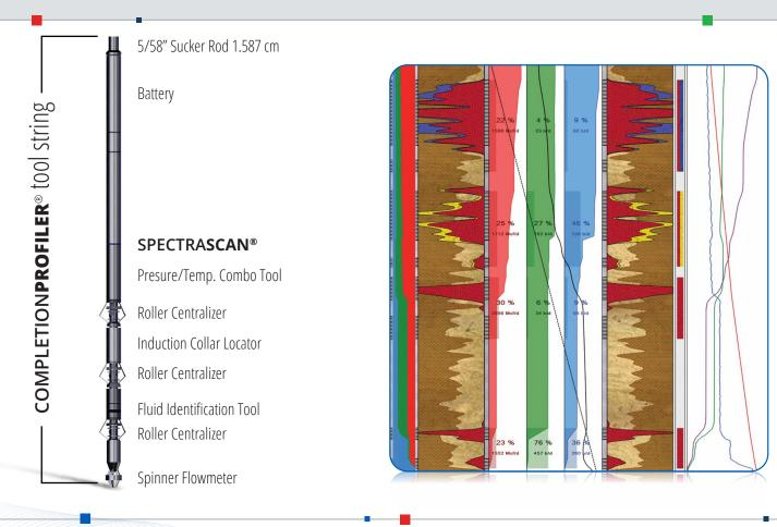
**COMPLETIONPROFILER**<sup>®</sup> utilizes a proprietary spinner design for adverse conditions, ensuring the highest data quality in high sand or debris environments and low velocity flow conditions. The rugged design ensures reliable operation in temperatures up to 350° F (176° C) and pressures up to 20,000 psi.
